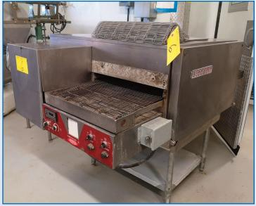
**BLODGETT** MT21-E DOUBLE STACK ELECTRIC CONVEYOR OVEN, 18" BELT, 28" TUNNEL, 120/240V, S/N 0792F0291101
