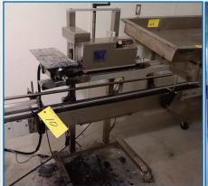
**STEELTEK** ST225/560/MKM HEAT SEALER W/ HITACHI PB-260U INKJET PRINTER
