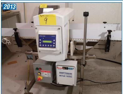
METTLER TOLEDO SAFELINE CON5460 FLOW-THROUGH METAL DETECTOR, 7" X 14" OPENING, S/N 119721
