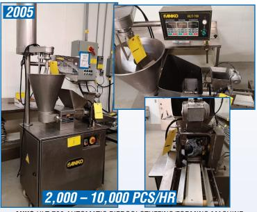
ANKO HLT-700 AUTOMATIC PIEROGI STUFFING/FORMING MACHINE W/ PIEROGI DIES, S/N 0506677, 220V, 60 HZ, 2,300W
